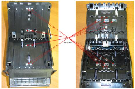
Be sure there is no dust accumulation, scratches or other mechanical damage.
